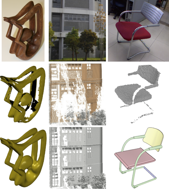
Figure 1: Surface reconstruction has grown in diversity in recent years resulting in techniques taking on specialized priors. ROSA [TZCO09], shown on the left, uses volumetric smoothness to aid in reconstruction. Non-local consolidation [ZSW*10], shown in the middle, uses global regularity in the form of structural repetition. Part composition [SFCH12], shown on the right, uses data-driven techniques.
