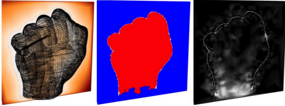
Figure 13: The approach of [?] first computes a robust unsigned distance function (left), and constructs an interior/exterior labeling (middle), and associated confidence (right) of the labeling. Note that low confidence is associated with regions of missing data, such as the bottom of the scan.
