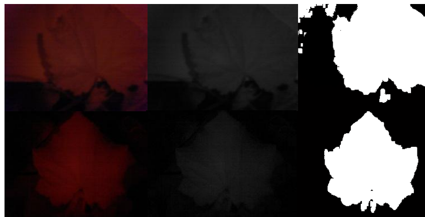
(a) Original near infrared image (b) Image with wavelet transform (c) Near infrared binary image using watershed algorithm
