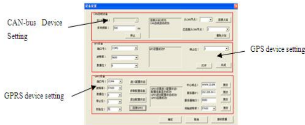
Fig.12 Interface of device settings
