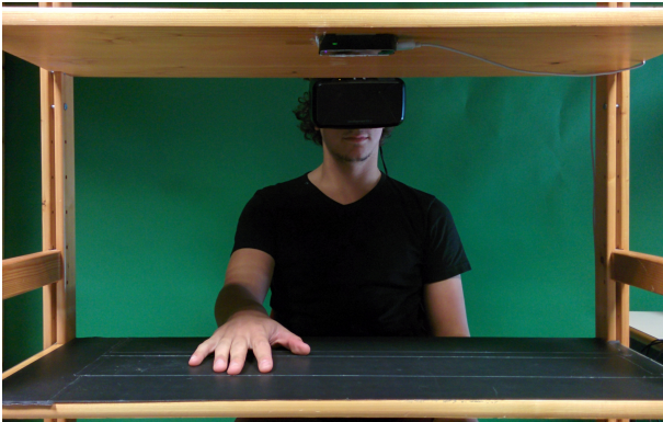
Figure 4: Experimental Setup. The interaction space was constrained by the shelf, which ensured an optimal tracking space for the Leap Motion (top). In addition, the bottom shelf provided passive haptic feedback.
