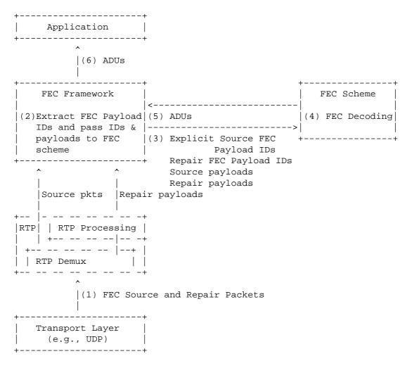
Figure 5: Receiver Operation with RTP Repair Flows
