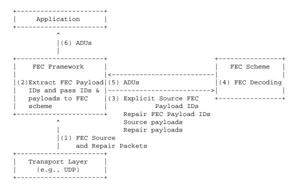
Figure 4: Receiver Operation with Sliding Window FEC Codes
