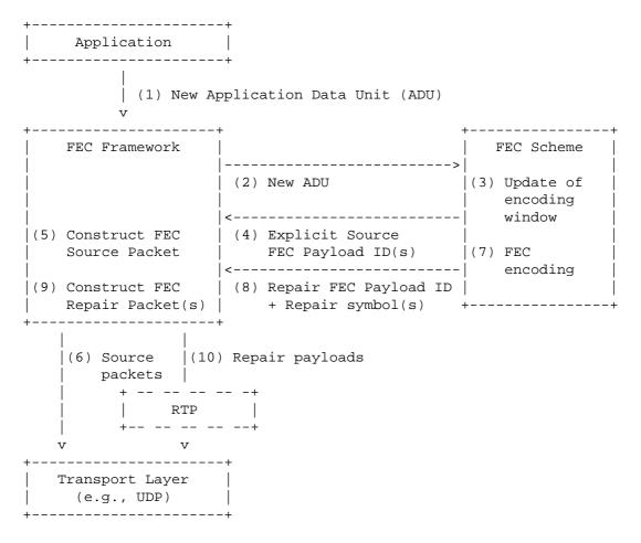
Figure 3: Sender Operation with RTP Repair Flows
