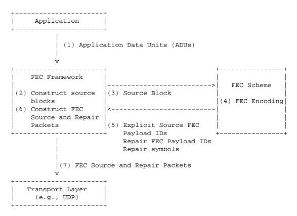
Figure 1: FECFRAME architecture at a sender.
