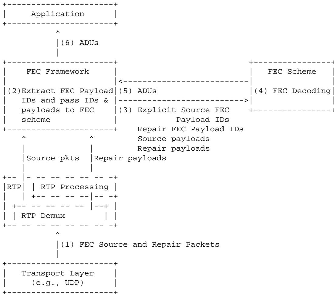
Figure 5: Receiver Operation with RTP Repair Flows
