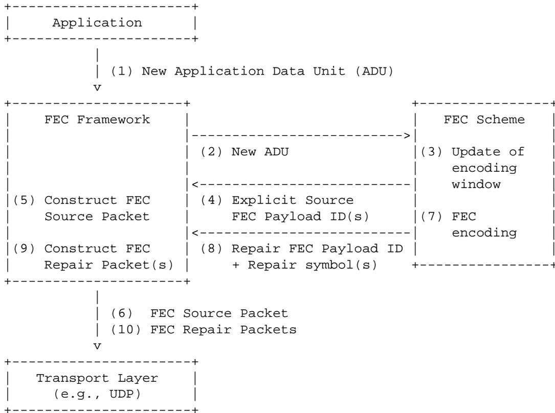
Figure 2: Sender Operation with Convolutional FEC Codes
