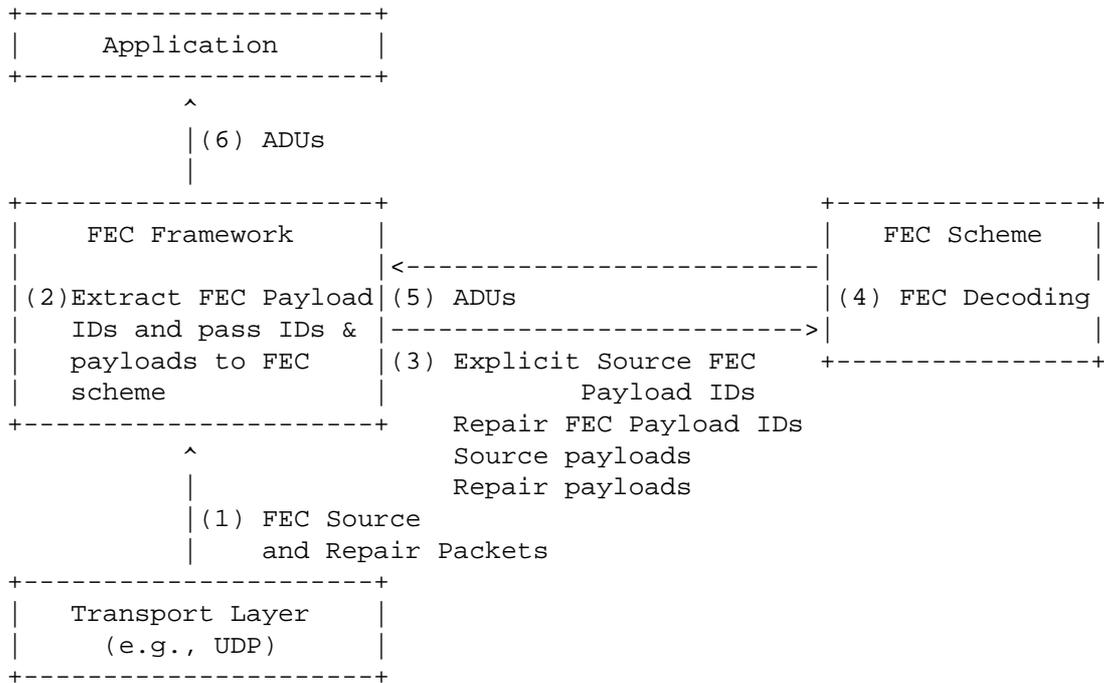
Figure 4: Receiver Operation with Sliding Window FEC Codes
