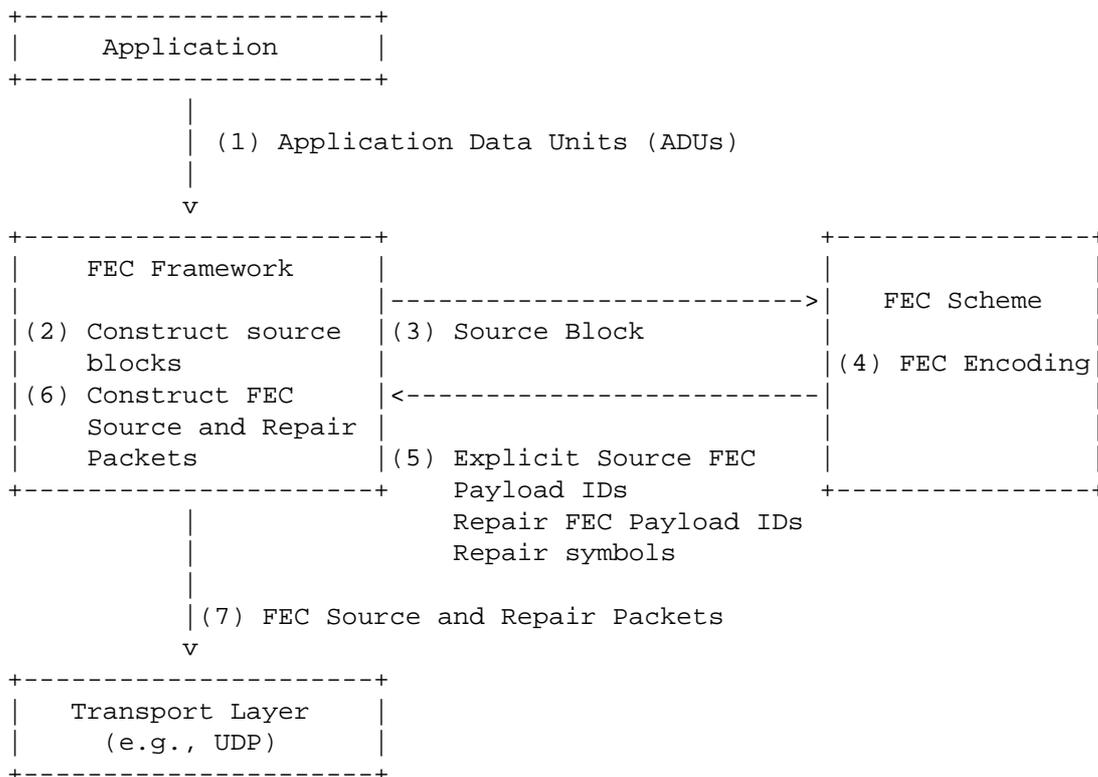
Figure 1: FECFRAME architecture at a sender.
