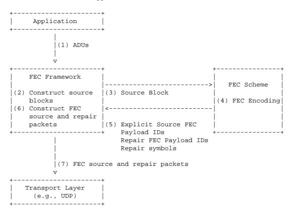
Figure 2: Sender Operation with Block FEC Codes
