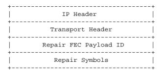
Figure 9: Packet Format for FEC Repair Packets
