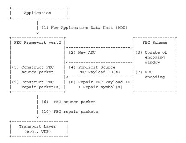
Figure 6: Sender Operation with Convolutional FEC Codes
