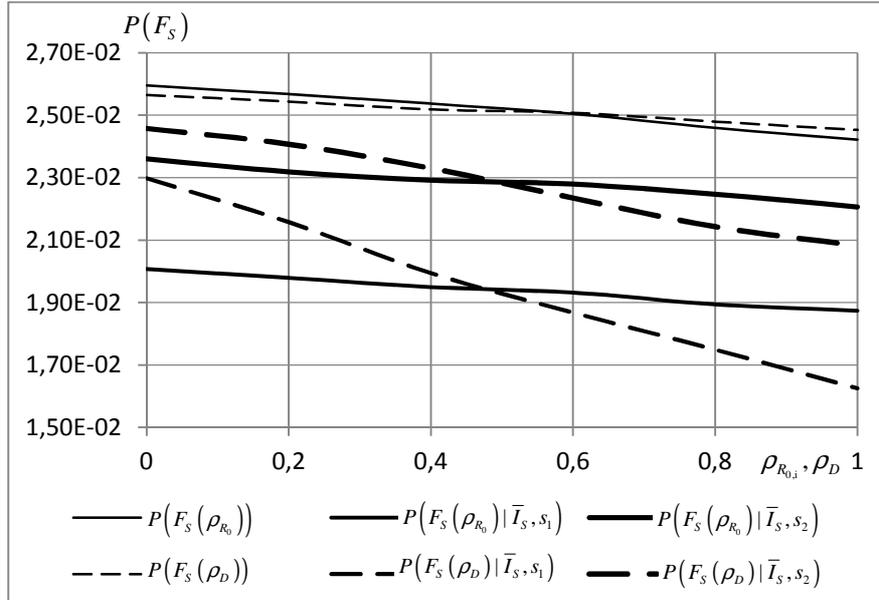
Figure 4: Prior and posterior system probability of failure ( $P(F_S)$  and  $P(F_S | \bar{I})$ ) in dependency of the resistance correlation, the damage correlation and the probability of component failure for different sensor positions.
