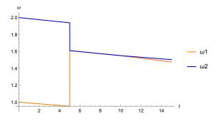
Figure 1: Simulation of the clutch model with resets. Mode change  $F \rightarrow T$  occurs at t = 5s and mode change  $T \rightarrow F$  occurs at t = 10s.
