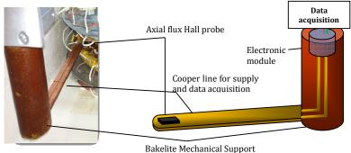
Fig. 4. Detail of the bakelite mechanical support for data acquisition.
