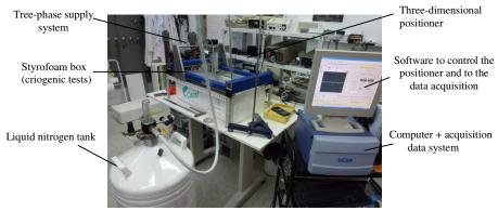
Fig. 1. Experimental apparatus for the static test of the HTS rotor.
