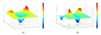
Fig. 7. Magnetic induction in half disc for a) tetrapolar e b) octopolar configurations, at liquid nitrogen temperature for  $I_m = 127$  A.
