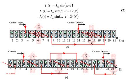
**Fig. 3.** Linear visualization of electrical connections, considering only phase 1, for a) bipolar configuration and b) tetrapolar configuration.
