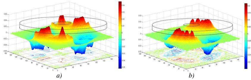
**Fig. 6.** Magnetic induction distribution, for tetrapolar configuration, *a*) due semi-stators supply, at room temperature and *b*) trapped in the rotor, after magnetization, at cryogenic temperature.
