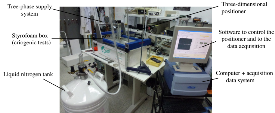
Fig. 1. Experimental apparatus for the static test of the HTS rotor.
