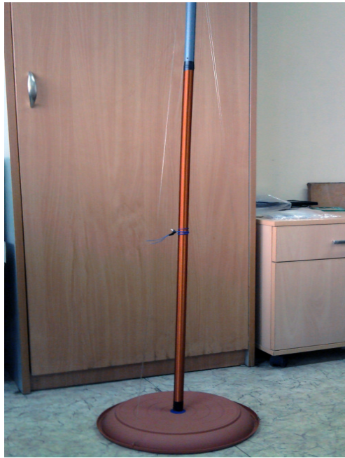
Fig. 1. Example of poorly constructed quarter-wave resonator coil.
