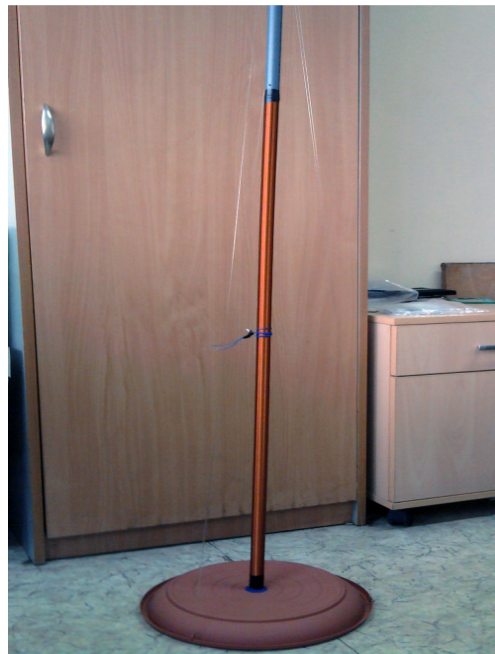
Fig. 1. Example of poorly constructed quarter-wave resonator coil.
