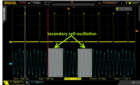
Fig. 3. Oscillogram of one of the driving channels of SG3525 and the response of the resonator.
