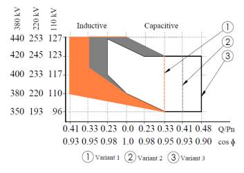
Fig. 3. Reactive power capability requirements for German case.
