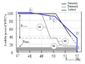
Fig.1. Power-frequency response required by mature grid codes in mainland networks.
