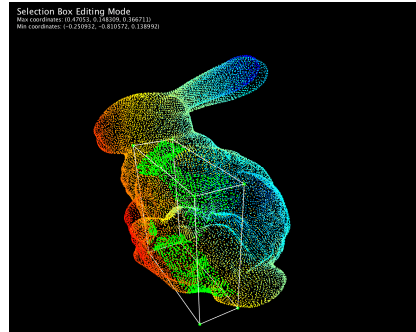
Fig. 3. Selection of points from a point cloud using a cuboid [6]
