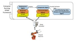
Fig. 4. PRIME Agent environment using a Semi-intelligent Resource
