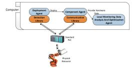
Fig. 5. PRIME Agent environment using a Passive Resource
