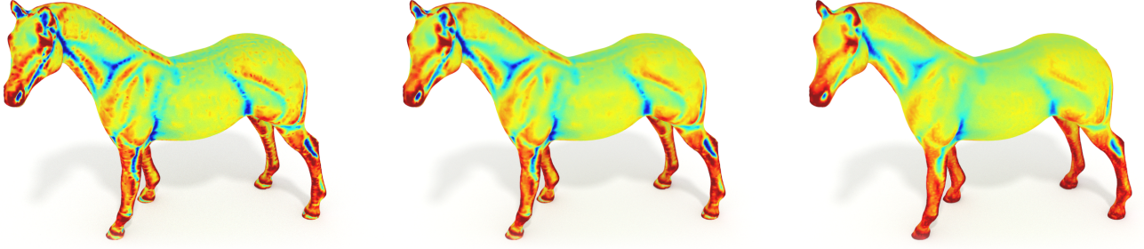
Figure 3: Mean curvature of the irregular horse mesh. (Left) the cotan formula [42] which is based solely on the mesh vertices, (middle & right) the 3-averaging formula (1), which additionally takes into account a normal at each vertex. For the middle image, the vertex normal is taken as the average of the face normals. In the rightmost example we smoothed the vertex normals before applying formula (1).
