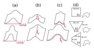
Figure 11: Validation experiment: We compare sounds obtained while varying three parameters: amount of compression (a),  $l_r$  (b) and  $l_c$  (c). We also measured the sounds obtained for 3 sheet shapes with the same compression,  $l_r$  and  $l_c$ : S1 is a square 10 cm x 10cm (d top); S2 is a trapezoid whose bases, of respective sizes 4cm and 16cm, are the curved borders (d middle); S3 is a trapezoid whose bases of sizes 4cm and 16cm, are the flat borders (d bottom).
