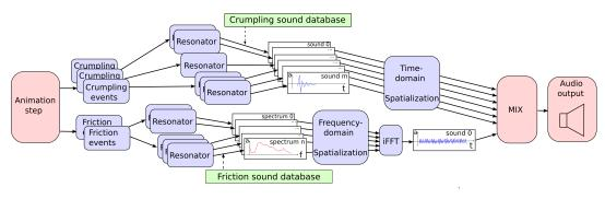
Figure 2: **Overview:** After computing the sound-producing events, each of them is associated with a set of *resonators*. Each of those *resonators* leads to a sound unit after querying it on a pre-computed sound data-base. Each sound unit is spatialized to adapt to our scene and the final resulting sound is obtained by mixing all the contributing sounds.
