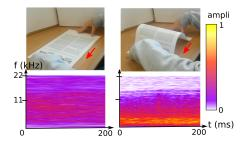
Figure 3: **Spectrogram of recorded friction sound** reveals slowly varying spectra in time, which is well approximated by a colored noise model. (left) Constrained friction sound obtained for a flat sheet of paper. (right) Unconstrained friction sound produced by a curved sheet.
