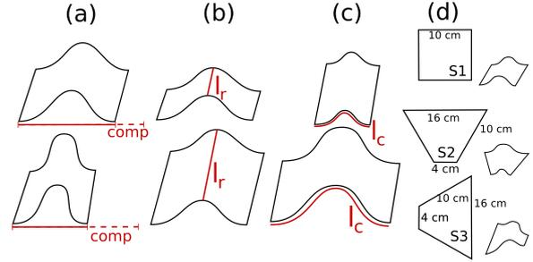
Figure 11: **Validation experiment:** We compare sounds obtained while varying three parameters: amount of compression (a),  $l_r$  (b) and  $l_c$  (c). We also measured the sounds obtained for 3 sheet shapes with the same compression,  $l_r$  and  $l_c$ : S1 is a square 10 cm x 10cm (d top); S2 is a trapezoid whose bases, of respective sizes 4cm and 16cm, are the curved borders (d middle); S3 is a trapezoid whose bases of sizes 4cm and 16cm, are the flat borders (d bottom).
