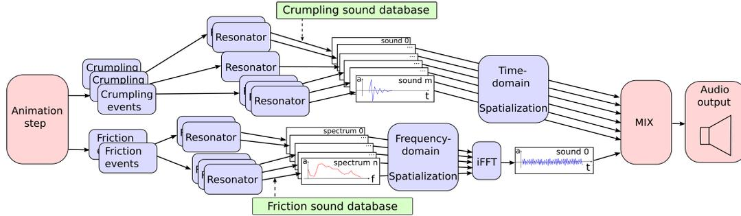
Figure 2: **Overview:** After computing the sound-producing events, each of them is associated with a set of *resonators*. Each of those *resonators* leads to a sound unit after querying it on a pre-computed sound data-base. Each sound unit is spatialized to adapt to our scene and the final resulting sound is obtained by mixing all the contributing sounds.
