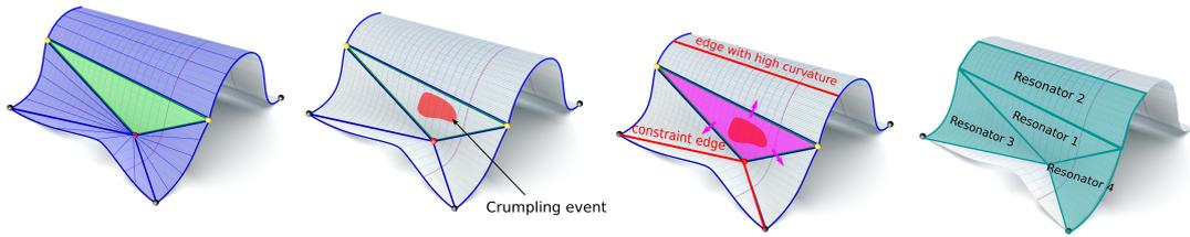
Figure 7: **Resonator estimation** (for a crumpling event): (left) curved and flat regions, (middle-left) detecting sound event, (middle-right) finding region of event and recursively finding the regions in which the vibrations can propagate, (right) resonators.
