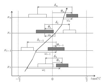
Figure 1: Problem notation. Green windows of the outbound direction of travel are shaded. Green windows in the inbound direction are in white. The travel speed trajectory and the basic notation is indicated only for the outbound direction for clarity.
