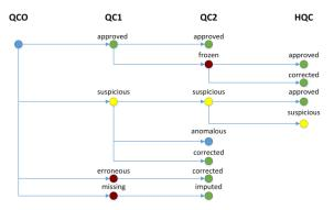
Fig. 3. Quality control of water consumption data.
