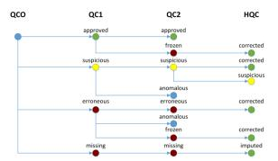
Fig. 2. Quality control of room temperature data.
