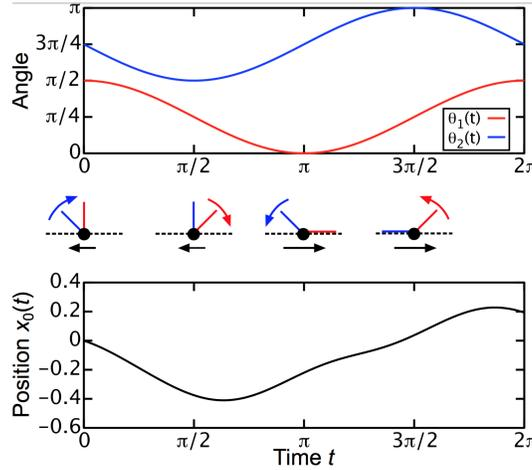
Fig. 2: Two legs oscillating sinusoidally according to  $\theta_1 = \pi/4 + a \cos t$  and  $\theta_2 = 3\pi/4 + a \cos(t + \pi/2)$ , where  $a = \pi/4$  is the amplitude. The second leg (blue) oscillates about  $\Phi_2 = 3\pi/4$ , while the first leg (red) oscillates about  $\Phi_1 = \pi/4$  with a phase lag of  $\pi/2$ . The swimmer position  $x_0$  translates about a fifth of the leg length after one cycle.
