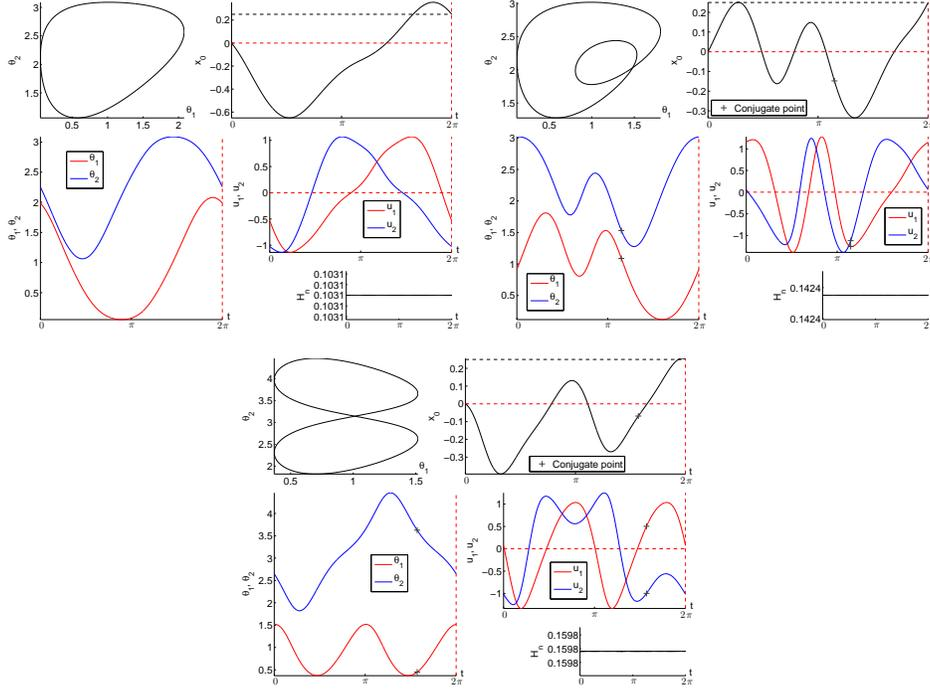
Fig. 5: Normal strokes : simple loop (left), limaçon with inner loop (right) and eight case (bottom). First conjugate points on  $[0, 2\pi]$  appear with a cross only for the limaçon stroke and the eight stroke.
