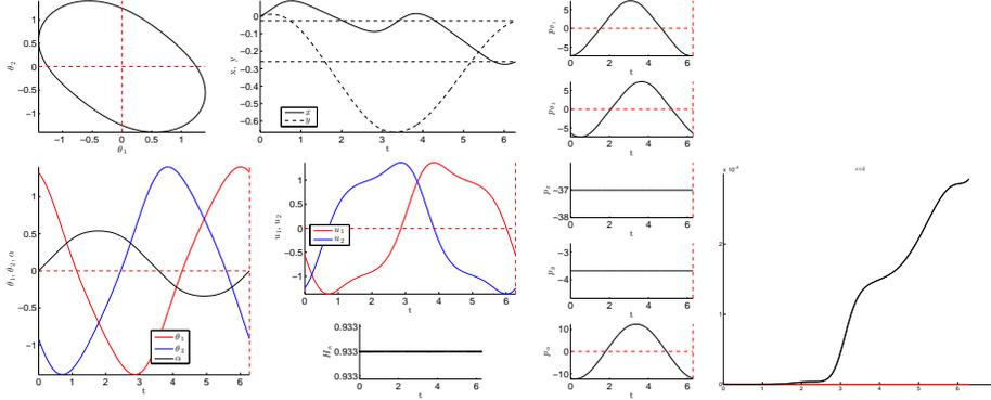
Fig. 16: (left) Simple loop stroke for the Purcell swimmer for the  $\int_0^T (u_1^2 + u_2^2)dt$  cost with  $T = 2\pi$ ,  $c_1 = 0.068$ ,  $c_2 = 0$  and imposing the periodicity on  $\alpha$ . (right) Test of conjugate points (no conjugate point on  $[0, 2\pi]$ ).
