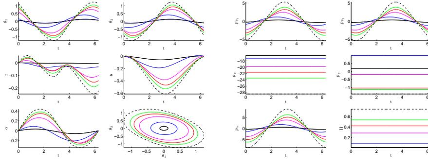
Fig. 15: One parameter family of simple loop strokes of the Purcell swimmer with the  $\int_0^T (u_1^2 + u_2^2)dt$  cost. The continuation is performed on the constant  $c_1$  where we fixed  $T = 2\pi$  and  $c_2 = 0$ .
