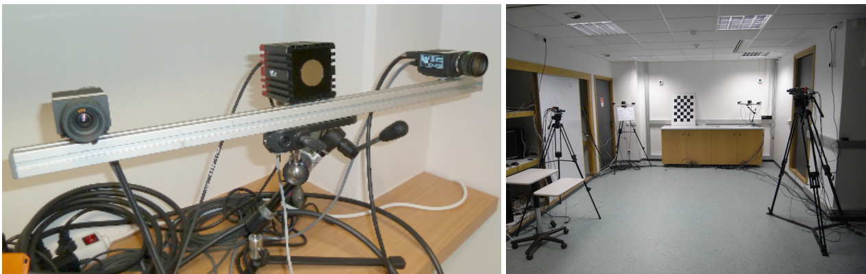
Fig. 13 A single system (left), comprising a time-of-flight camera in the centre, plus a pair of ordinary color cameras. Several (four) such systems can be combined together and calibrated in order to be used for 3D scene reconstruction (right).
