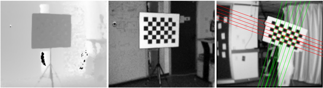
Fig. 12 The depth (left) and amplitude (middle) images of an OpenCV calibration pattern grabbed with an SR4000 camera. The actual image resolution is of 176 \times 144 pixels. The amplitude image (middle) has undergone lens undistortion using the model briefly described in section 6.3. The calibration pattern detected in the amplitude image (right) using the method of [Hansard et al., 2014].
