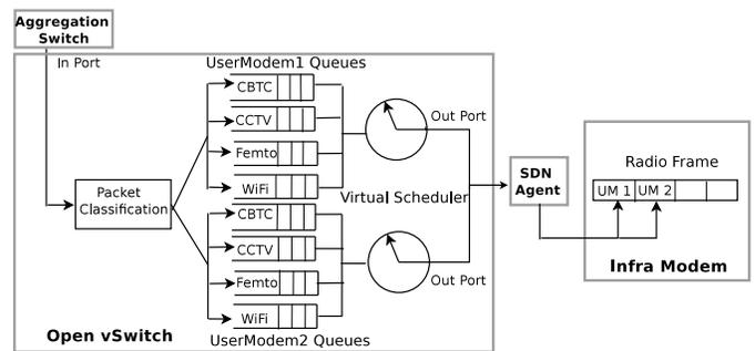
Fig. 3: Packet Scheduling using Priority Queuing in OVS.
