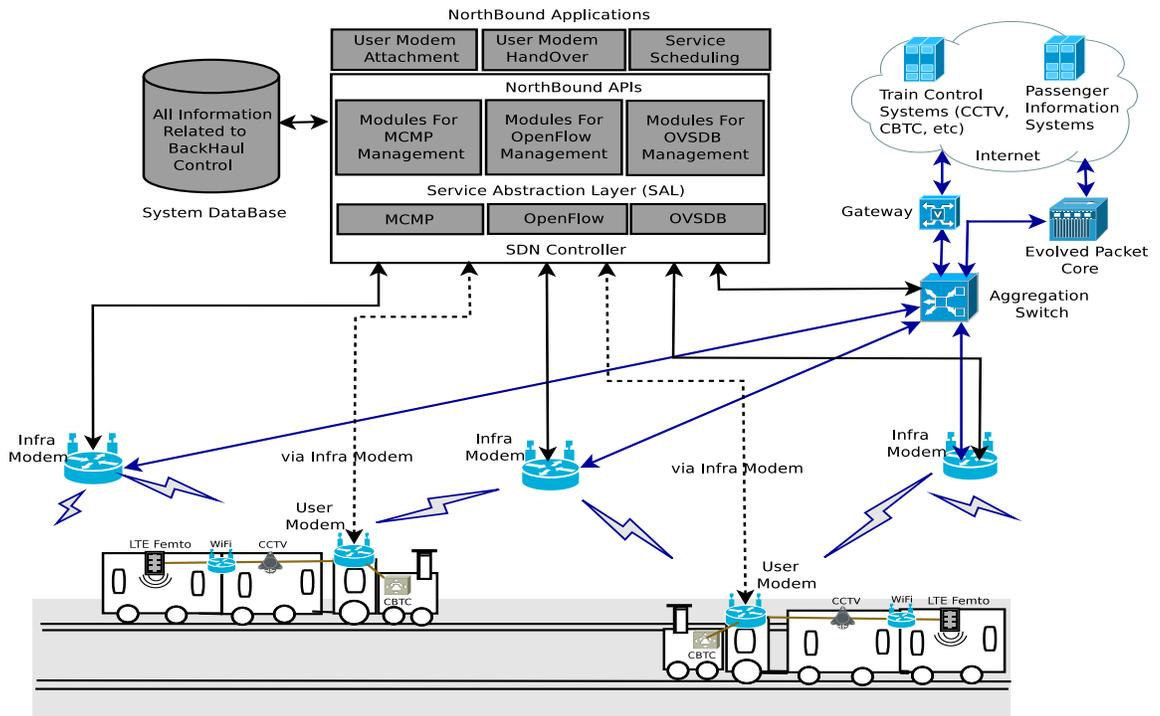
Fig. 1: Software Defined Mobile Backhauling for TWC Architecture.
