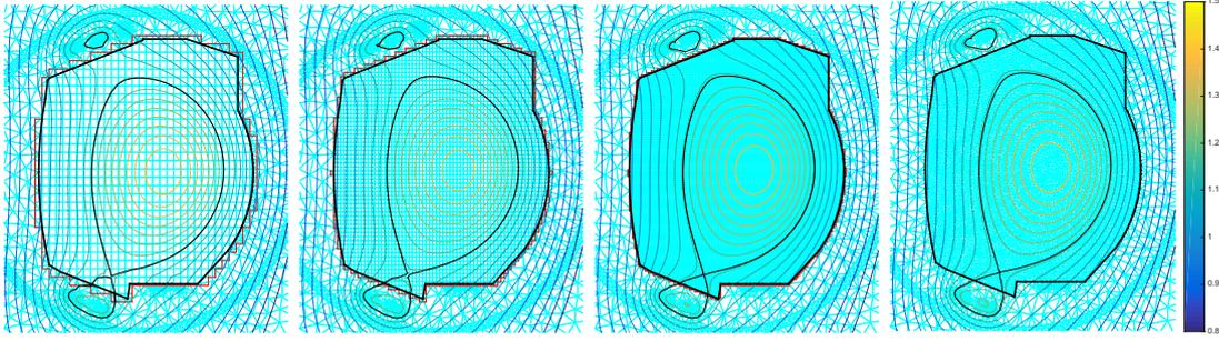
Figure 3: Contour plots of the solution by the MEM (13) and Bogner-Fox-Schmit elements (BFS) for an increasing number of elements in the interior rectangular mesh  $\tau^{\text{in}}$  (1st, 2nd and 3rd from the left) and a reference solution without MEM but with linear Lagrangian finite elements.
