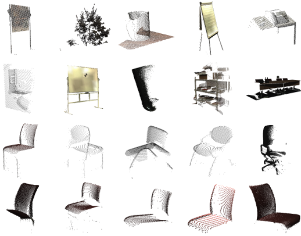
Figure 5: Indoor objects. We acquired 20 indoor objects with a Leica Scanstation P20 laser scanner. The sampling of the objects is heterogeneous and partly suffers from anisotropy. The lower 10 objects are labeled as chairs whereas the upper ten objects are labeled as non chairs.
