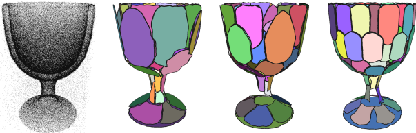
Figure 1: Multiscale Planar Abstraction. Left: Input point cloud of a goblet with outliers and noise. Mid to Right: Planar abstraction with varying fitting tolerance from coarse to fine: 1%, 0.5% and 0.25% of bounding box diagonal.
