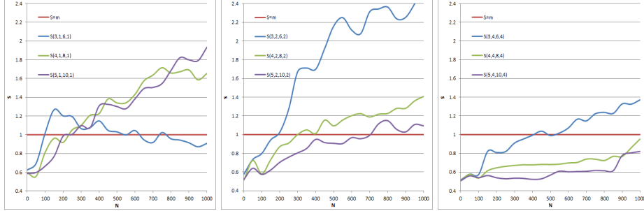
Fig. 5. Scaling speedup with doubled number of VMs v , each with 1 (left), 2 (middle), and 4 CPU cores (right)
