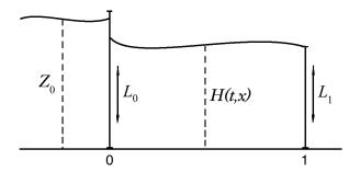
Fig. 1. Water channel with two spillways
