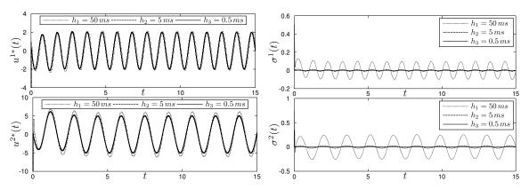
Figure 2: Time evolution of the control input  $u_k = u_k^{\text{nom}} + u_k^{\text{sv}}$  (left) and the associated sliding variable (right), for the sampling times  $h \in \{50 \, ms, 5 \, ms, 0.5 \, ms\}$ .
