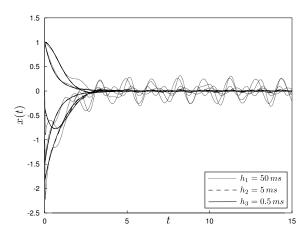
Figure 3: Time evolution of the piecewise linear trajectories x(t) of the discrete-time system (61) for the sampling times  $h \in \{50 \, ms, 5 \, ms, 0.5 \, ms\}$ .
