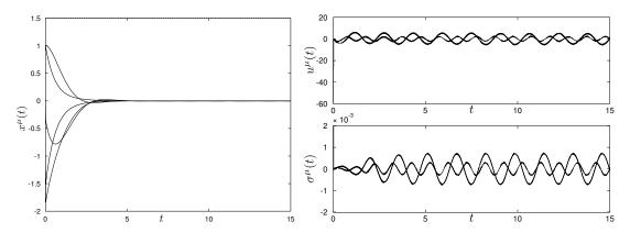
Figure 1: Time evolution of the control input  $u = u^{\text{nom}} - K\sigma - \gamma(z)\mathcal{M}^{\mu}(\sigma)$  and the corresponding system trajectories and sliding variable with  $\mu = 0.001$ .
