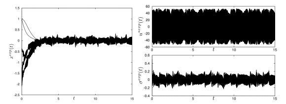
Figure 4: Time evolution of the control input  $u = u^{\text{nom}} - K\sigma - \gamma\sigma/(\|\sigma\| + 0.001)$  and the corresponding system trajectories and sliding variable with a sampling step h = 5ms.
