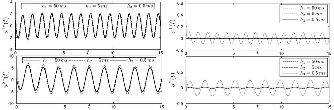
Figure 2: Time evolution of the control input  $u_k = u_k^{\text{nom}} + u_k^{\text{sv}}$  (left) and the associated sliding variable (right), for the sampling times  $h \in \{50 \text{ ms}, 5 \text{ ms}, 0.5 \text{ ms}\}$ .
