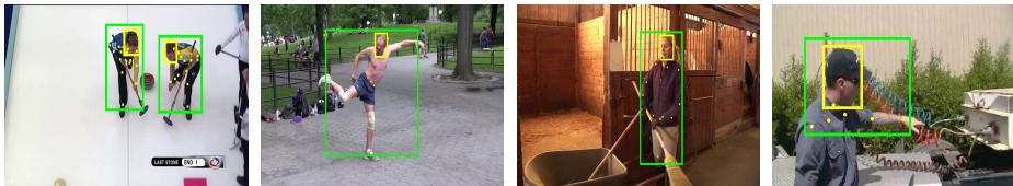
Fig. 3. Examples of bounding boxes (green) estimated from annotated joints and head (yellow) on the MPII Human Pose dataset.
