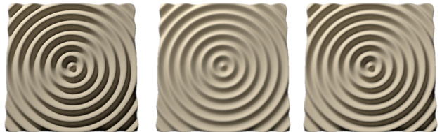
Figure 6: Light size. With a fixed distance of 5 diameters, too small (a) or too large (b) light sizes tend to remove or hide important shape details. Our suggestion (c) produces soft shadows while preserving main tonal variations.
