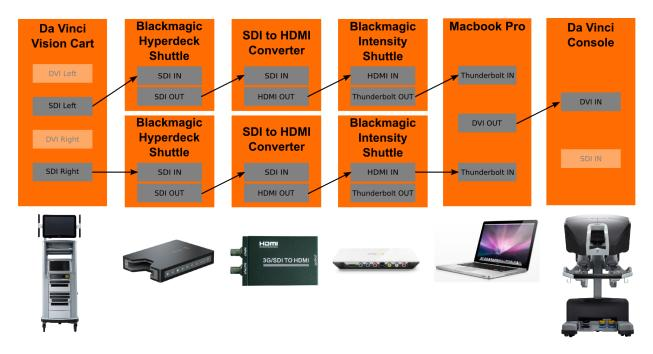
Fig. 3. Hardware setup for Per-operative Liver registration.
