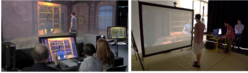
Figure 4: Our VR rehearsal sample environment running in a large-screen immersive room and on a portable projection screen: the actor rehearses the scene under the supervision of the technical team.
