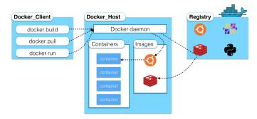
Figure 1. High-level overview of Docker architecture.
