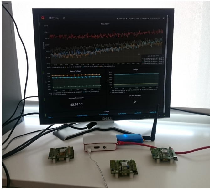
Fig. 3. The setup of the PEACH demonstration, including the motes, the manager and the web interface of the back-end system.
