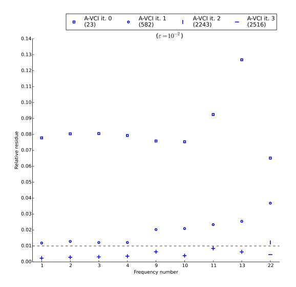
FIG. 3. Convergence curves of the H<sub>2</sub>CO active frequencies with an IR intensity larger than 2 km/mol and the highest one  $\nu_{22}$  computed with the A-VCI Algorithm 1 ( $\varepsilon = 10^{-2}$ ). The y-axis represents the relative residue and the x-axis the frequency number. For each iteration j the size of the subspace  $B^{(j)}$  is given in parentheses.
