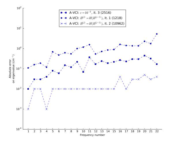
FIG. 4. Absolute error (logarithmic scale in cm<sup>-1</sup>) of the A-VCI frequencies computed for H<sub>2</sub>CO with respect to the calculation in the reference basis (see Table I). The size of the subspace  $B^{(j)}$  at iteration j is given in parentheses. We compare results obtained with the enrichment strategy (12)  $(B^{(j)} = H(B^{(j-1)}))$  at iteration 1 and 2 and with the Algorithm 1 ( $\varepsilon = 10^{-2}$ ) at iteration 3.
