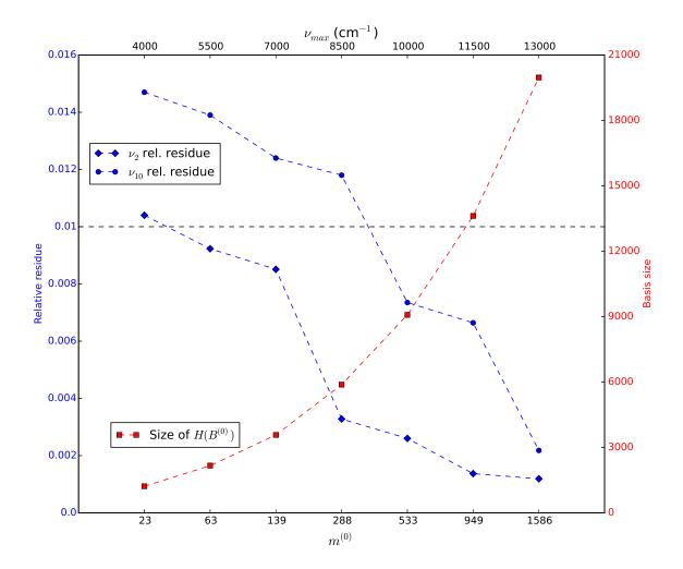
FIG. 2. Relative residue (blue curves) and corresponding  $H(B^{(0)})$  basis size (red curve) as function of the size  $m^{(0)}$  of  $B^{(0)}$ . The frequency  $\nu_{max}$  (cm<sup>-1</sup>) corresponding to  $m^{(0)}$  is reported on the upper axis. The residue is represented for  $\nu_2$  and  $\nu_{10}$  computed in  $H(B^{(0)})$ .
