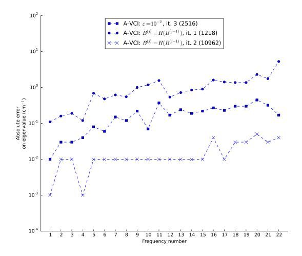
FIG. 4. Absolute error (logarithmic scale in cm<sup>-1</sup>) of the A-VCI frequencies computed for  $H_2CO$  with respect to the calculation in the reference basis (see Table I). The size of the subspace  $B^{(j)}$  at iteration j is given in parentheses. We compare results obtained with the enrichment strategy (12)  $(B^{(j)} = H(B^{(j-1)}))$  at iteration 1 and 2 and with the Algorithm 1 ( $\varepsilon = 10^{-2}$ ) at iteration 3.
