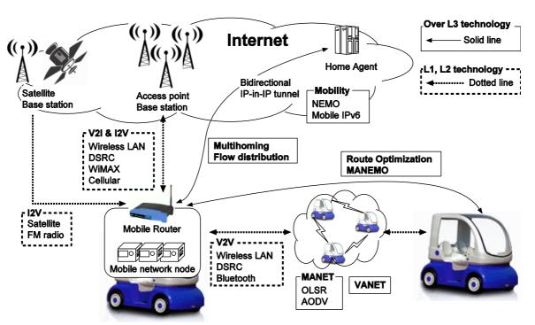
Figure 1: Overview of the application of network technologies in the vehicle domain
