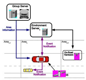
Figure 2: P2P/Cellular network overlay network for vehicular communications
