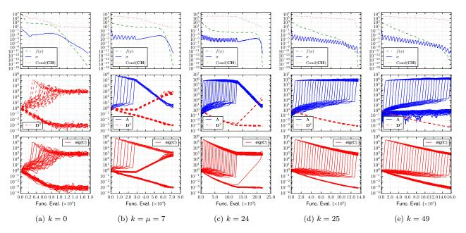
Figure 3: Single run results of VkD-CMA with k = 0, 7, 24, 25, 49 on  $f_{\text{TwoAx}}$  in 50 dimension. The best function value at each iteration, the step-size  $\sigma$  (on the top), the condition number Cond(**CH**), each element of **D** and **A** (on the middle), each eigenvalue of  $\mathbf{C} = \mathbf{D}(\mathbf{I} + \mathbf{V}\mathbf{V}^{T})\mathbf{D}$  (on the bottom) are shown.
