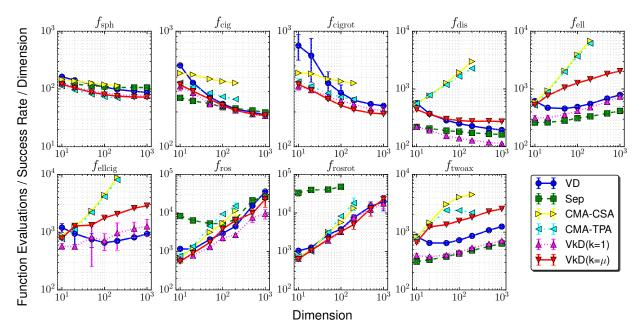
Figure 2: Function evaluations to reach the target value averaged over the successful runs divided by the success probability and the dimension. Each error bar shows the standard deviation.
