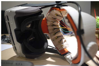
Figure 3: Prototype of a HMD device that directly embeds EEG electrodes – here a Vrvana Totem a . Picture © Alexandre Girardeau.
