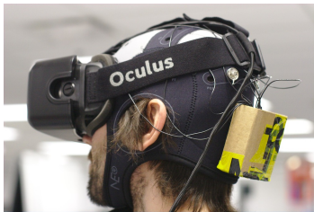
Figure 2: The Oculus Rift DK1 HMD a is combined with Neuroelectronics Enobio EEG cap b and OpenBCI amplifier c to both immerse and monitor user's brain activity.
