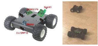
Figure 4. The cooperating robots during an experiment.
