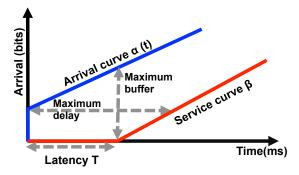
Fig. 3. Arrival curve, service curve, delay bound
