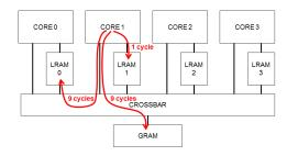
Fig. 1. Microcontroller architecture used in the challenge
