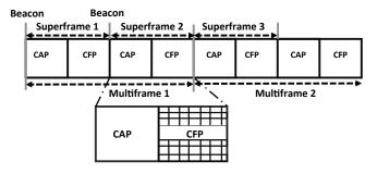
Fig. 1. Multi-frame structure of DSME
