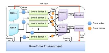
Fig. 1. Run-time monitoring reference architecture [4].
