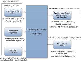
Fig. 1. Inputs/Outputs of the Framework
