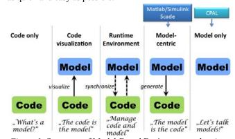
Figure 1: Spectrum of Model-Based Design approaches (core of the figure from [Br04]).
