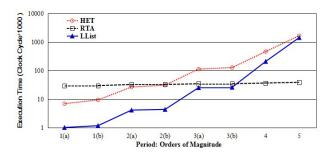
Fig. 1. Average execution time required by the HET, RTA, and LList-based exact schedulability tests versus number of orders of magnitude range of task periods. The range of periods starts from 10 and 10<sup>4</sup> for (a) and (b), respectively. Note both x and y-axes are logarithmic scales.
