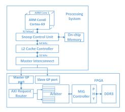
Fig. 1. Predictable SoC architecture
