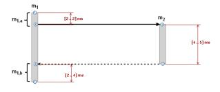
Figure 2: Synchronous call between two operations in the TEMPO Design pivot model
