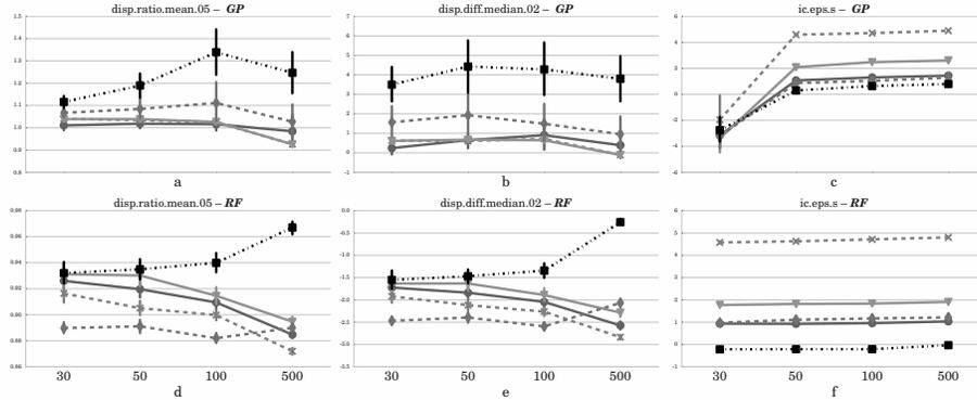
Fig. 4: Values of 3 features vs initial sample size  $s$ , for the 5 test functions ( $d = 20$ ), using a surrogate model (GP for (a,b,c), RF for (d,e,f) ) to add  $s' = 2000$  points to the sample set.
