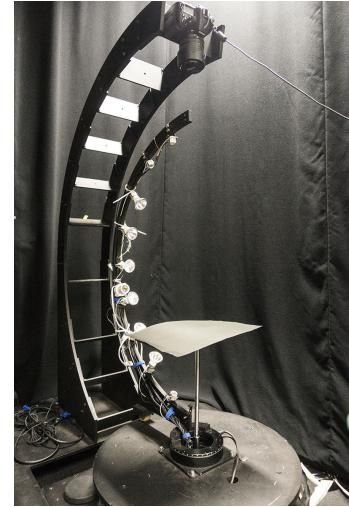
Figure 2: Our acquisition platform: the sample and camera are static and aligned with each other, the light arm rotates around them. Arm position and picture acquisition are controlled by a computer.
