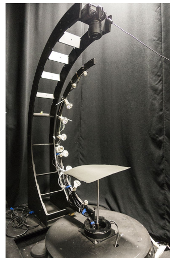
Figure 2: Our acquisition platform: the sample and camera are static and aligned with each other, the light arm rotates around them. Arm position and picture acquisition are controlled by a computer.
