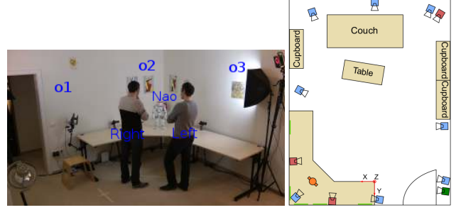
Fig. 2. The Vernissage setup. Left: Global view of the “exhibition” scene showing wall painting, two persons and the NAO robot. Right: Top view representation of the room.
