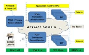
During normal operation on a full hardware configuration, the GTL system's network CPU contained the Network & Front End module, the next CPU contained the Application Control part, and the remaining two CPUs contained one SIBAS DBMS system each. For communication between the CPUs, a mini version of the previously mentioned Nordnet was used.
