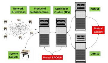
Two pairs of CPUs were mutual backup for each other. In normal operation one CPU interfaced to the NSB network, the next one contained all application programs, and the remaining two CPUs were both database machines. The database machines split the database between themselves in order to share the load, and trains would literally move between the database machines as they moved along the rail network in real life.
