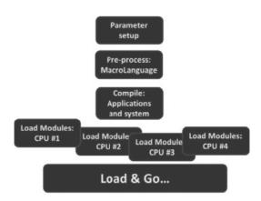
The output of the system builder was load images for each of the CPUs at hand, and the total system was initiated by loading the CPUs and typing the "initialize" command on the system console.
